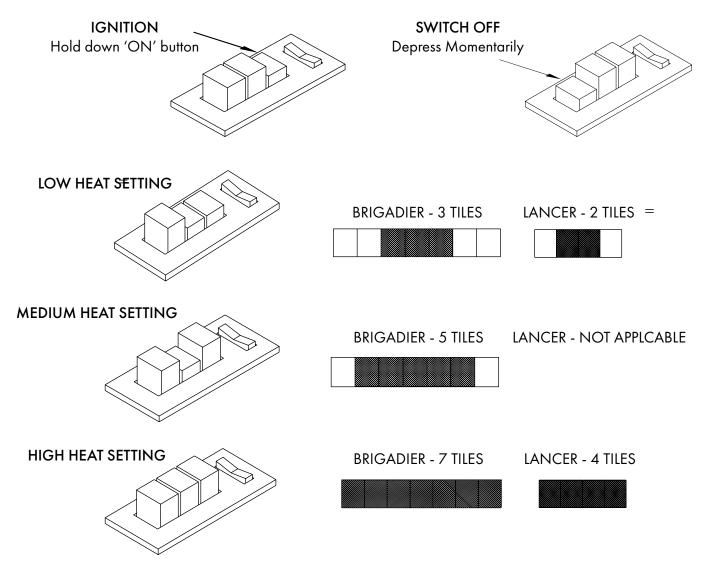
Low, medium and high settings can be obtained by setting the buttons set as shown in the diagrams above. If you depress the button firmly and it remains in the half way position, a second depression will return it to the fully up position.
