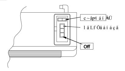
The ON/IGNITION/LOW button and the MEDIUM/HIGH button each have two operating positions, which provides three heat settings.
